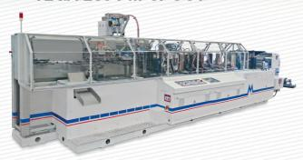
VEGA 285 PM-SPOUT machines are dedicated for Angular or Linear Spout fixing. Option available to make Three Side Seal and Stand up pouches with Zipper is possible on same machine without Spout.
